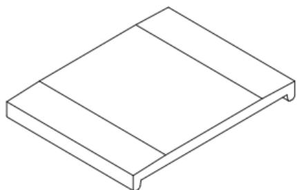
THRAIL-DB2 resilient pad is made of wear-resistant durable thermoplastic which has elastomeric properties..This material is immune to oil,grease and ultraviolet light.They have been tested to many times the design loads and show complete recovery. Tapered leading and trailing edges along the rail reduce edge loading on the sole plate and grout when
