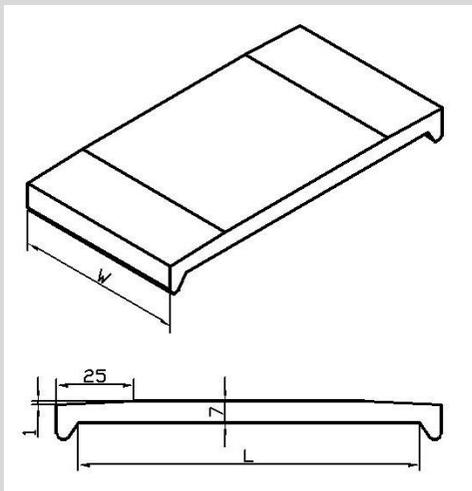
THRAIL-MK2 Resilient Pad For Discontinuous Rail Support
