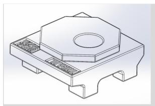
The THRAIL-HS2420 through-bolted clips(punched clips) are more convenient and efficient in installation.They are more economical in cost than welded
