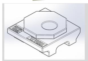
The THRAIL-HS2015/21 through-bolted clips(punched clips) are more convenient and efficient in installation.They are more economical in cost than welded
